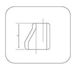
The function of both types of reducer is to reduce the line from a larger to a smaller pipe size, this obviously results in an increased flow pressure.
