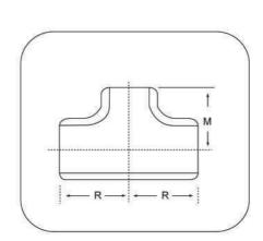
The Reducing Tee is manufactured with the branch outlet smaller than the run to obtain the desired flow and pressure through the system.
