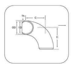
distance and is equivalent to the radius through which the elbow is bent.
