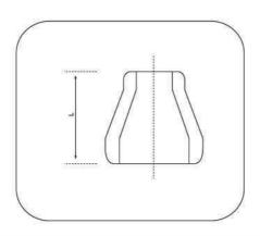
The Concentric Reducer is so manufactured that both inlet and outlet ends are on a common centre line. The Concentric reducer is easier and less expensive to produce but does not allow quite the same versatility as the Eccentric Reducer. The lengths of both types are fixed by manufacturing standards.
